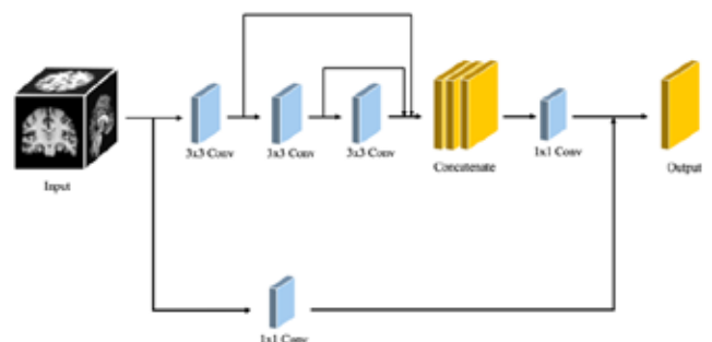
Fig 2. The convolution block of registration network in our model. Each block consists of three 3x3 convolution blocks for multi-scale and two 1x1 convolution blocks to reduce number of channels.
