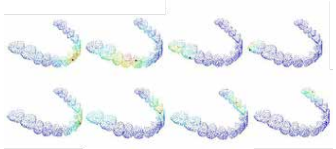
Fig.3 The point-wise attention map for different query points (indicated by •), rainbow color range (blue to red) indicating increasing attention weight
