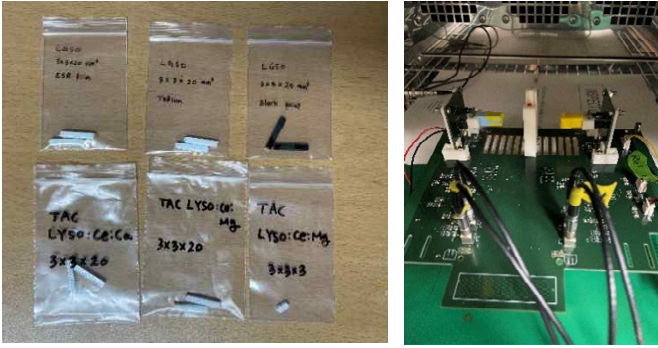
Figure 2. Tested Scintillation Crystals (left), Coincidence Event Data Acquisition Setup (right)
