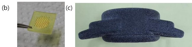
Fig. 2. Microneedle system: (a) Illustration of the system, (b) Microneedle Array and (c) Wearable Fluorescence Detecting Sensor
